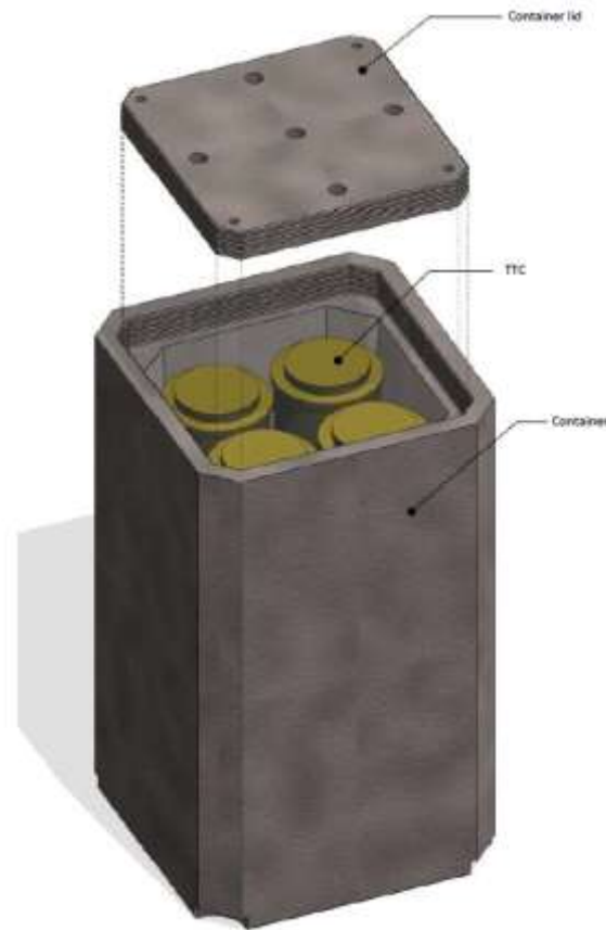
Figure 5-6 3-D view of disposal container [26].
